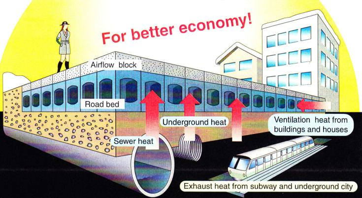
This snow melting system utilizes unused heat from sewers, ventilation heat from buildings and houses, exhaust heat from the subway and underground city, and underground heat. The system transfers the heat to a hollow space in a roadbed and then to the ground through airflow blocks to melt snow. Melted snow is discharged through the airflow blocks to the underground or drainage facilities.
